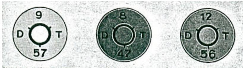
Common Cartridge                      Armor Piercing Cartridge                      Tracer Cartridge
